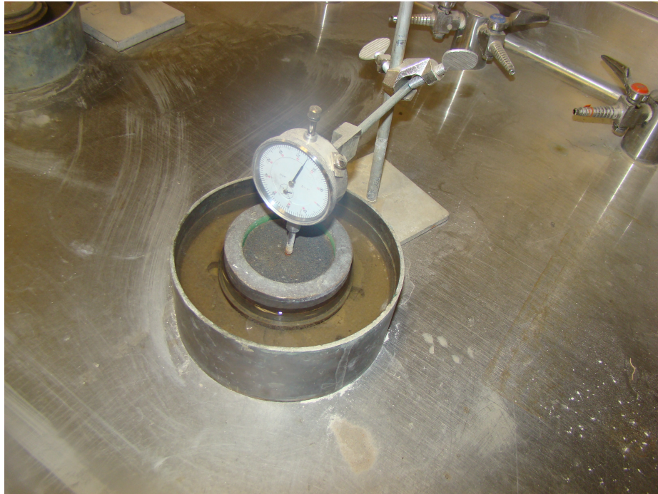
Figure 4.5 Laboratory Setup of One Dimensional Free Swell Test
