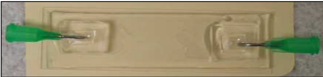
Figure 11: Global view of the microfluidic device with the input and output ports connected.
