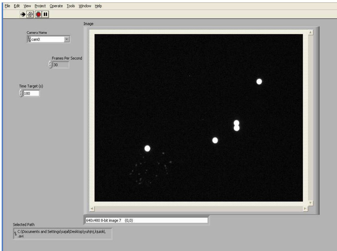
Figure 19: Front panel of LABVIEW VI for acquiring images of flowing beads, cells and fluorescein.
