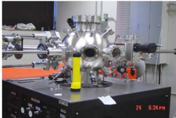
Figure 3.3 Side view of PLD system.
