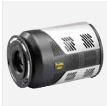
Figure 2.16: Pixis 400BR Focal Plane Array
