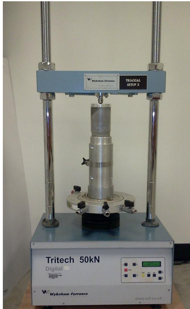
Figure 3.9 Cylindrical mold mounted on Triaxial Loading Frame
