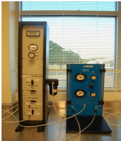
Figure 3.7 Pressure control panels
