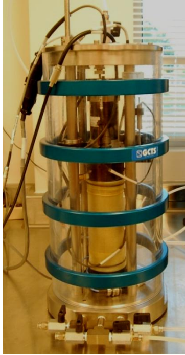
Figure 3.4 Proximator-based RC Main cell
