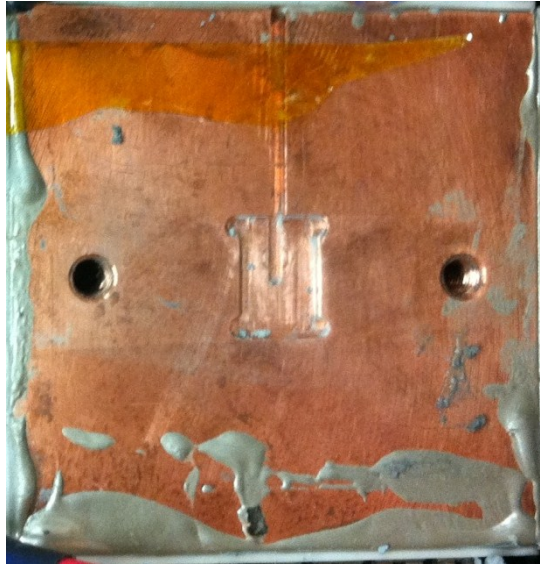
Figure 5.8 Bottom Surface of Copper Core Showing Recess Portion for Chip Resistor and Thermocouple
