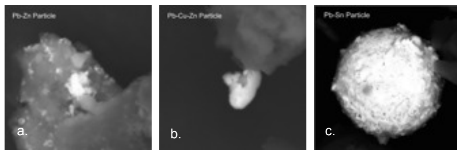
Figure 3.3 Pb-bearing particles of various forms: small dispersed in Zn-bearing matrix (a) small composed of Pb-Cu-Zn (b), spherical composed of Pb-Sn (c)
