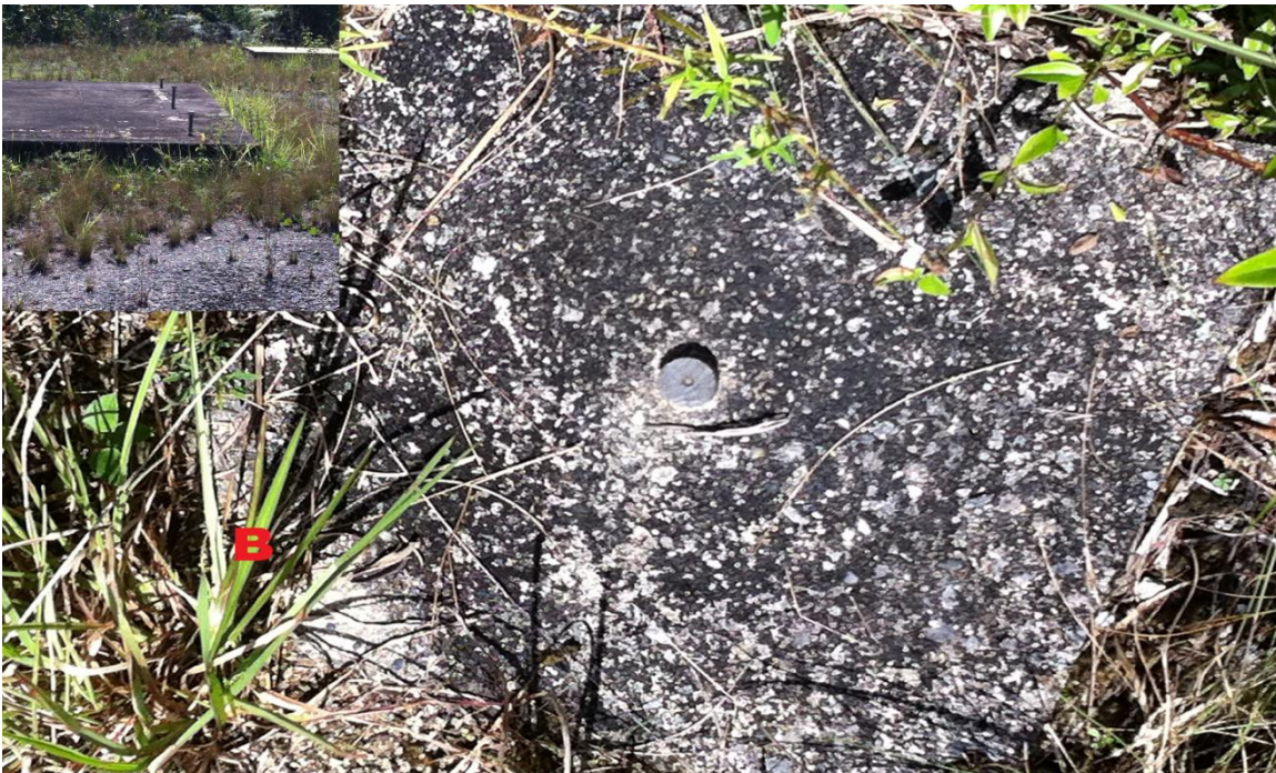
Figure A3. Photographs of site ARC2 acquired during May 2011 campaign. (A) Photoview facing south. (B) Geodetic monument at ARC2. The pin is epoxied into concrete adjacent to the helipad.
