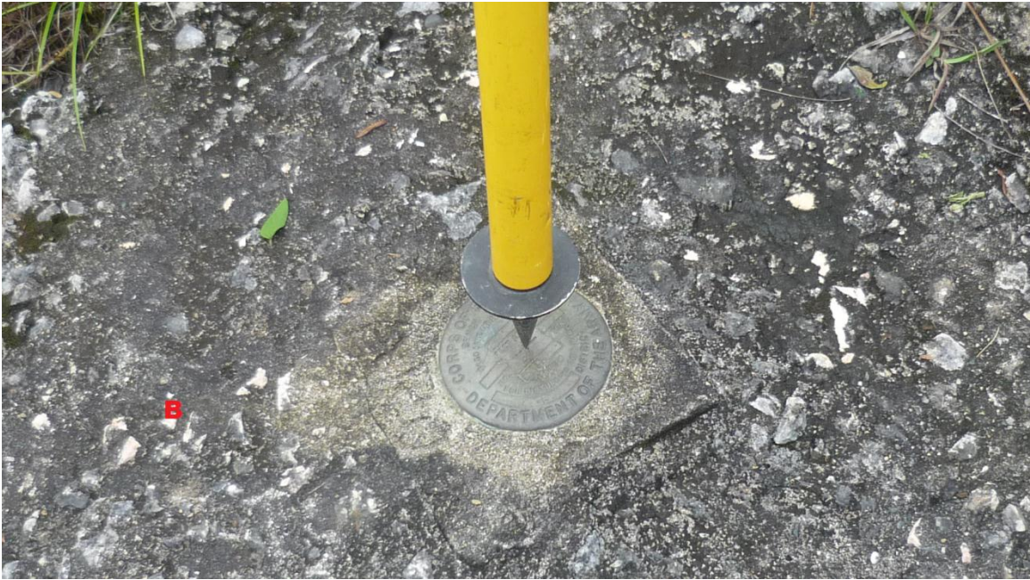
Figure A2. Photographs of site ARC1 acquired during May 2011 campaign. (A) Photoview facing west. (B) Geodetic monument at ARC1, the geodetic benchmark is inside a concrete slab cemented into local bedrock.
