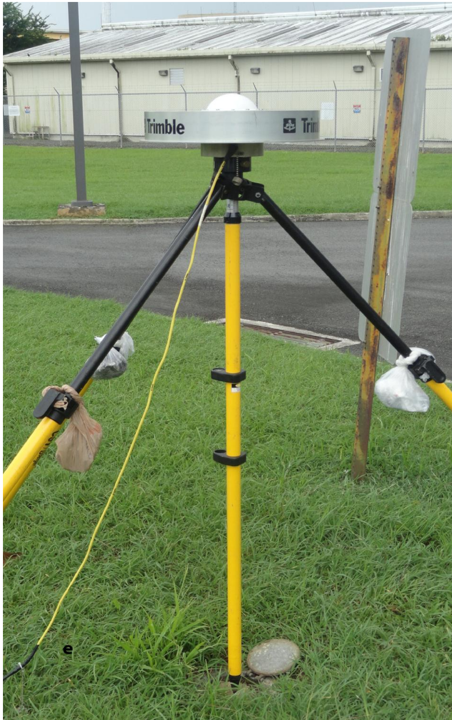
Figure 2.3 GPS geodetic antenna - standard tetrapod with choke ring antenna.
