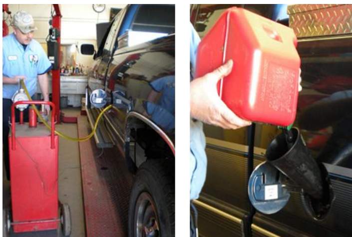
Figure 3.7 The fuel tank being drained and replaced with another fuel
