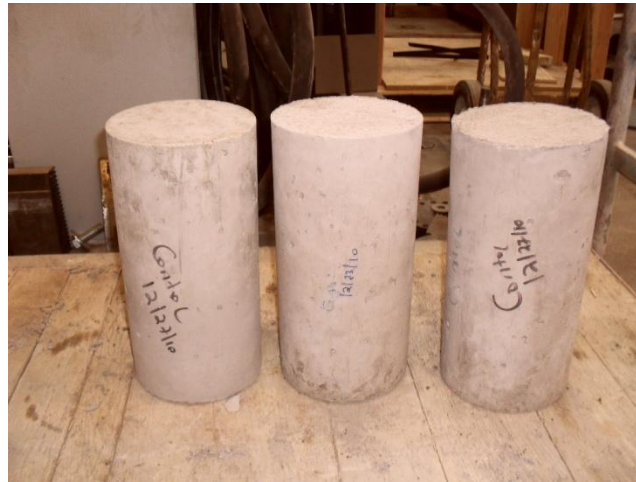
Figure 7.2: Control Concrete (No TDA) after exposure to 200°C for 3 hrs, no noticeable cracks or spalling was observed.
