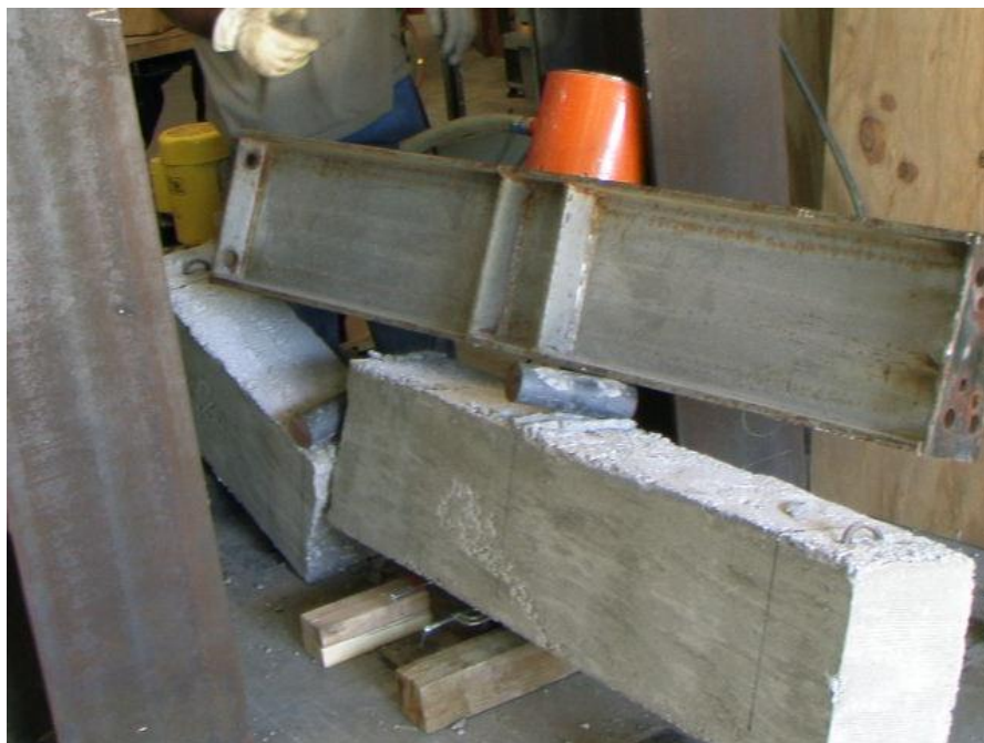
Figure 8.30: Experimental Results for the Crumb concrete (7.5%Crumb) Beam
