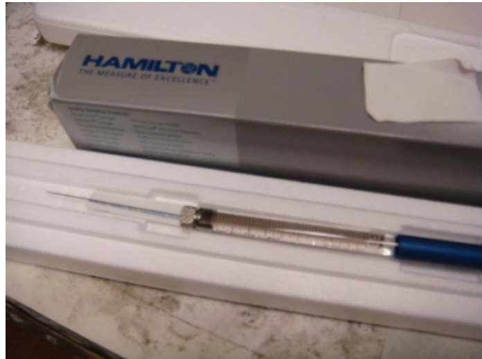
Figure 3.18 Apparatus for liquid characterization (a) Sample before and after being centrifuged, (b) Sample after dilution, (c) Hamilton 5 \mu L syringe
