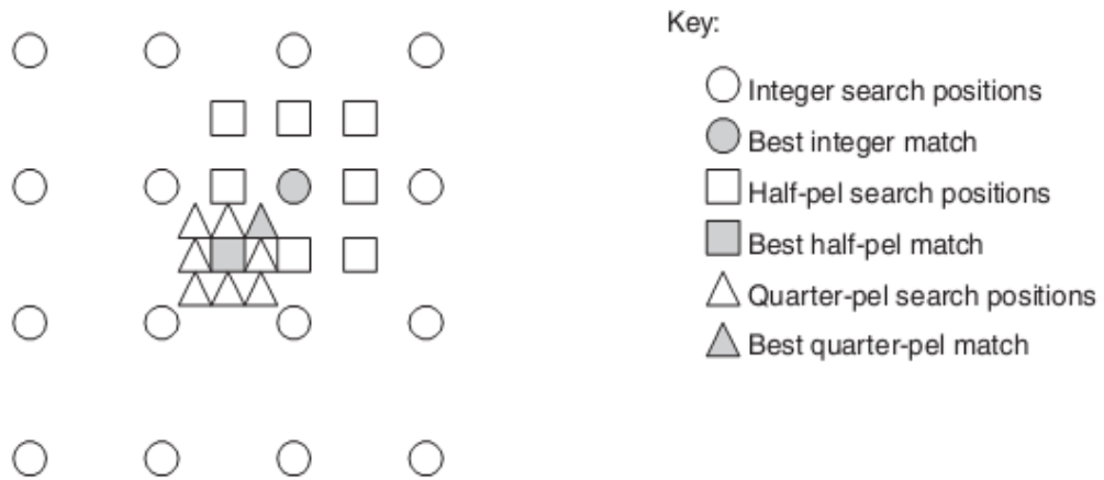
Figure 2.11 Integer, half-pixel and quarter-pixel motion estimation [11]
