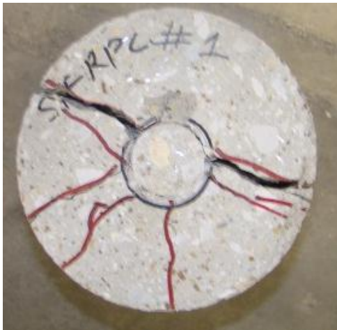
Figure 3.43 Typical Photos from Double Punch Test
