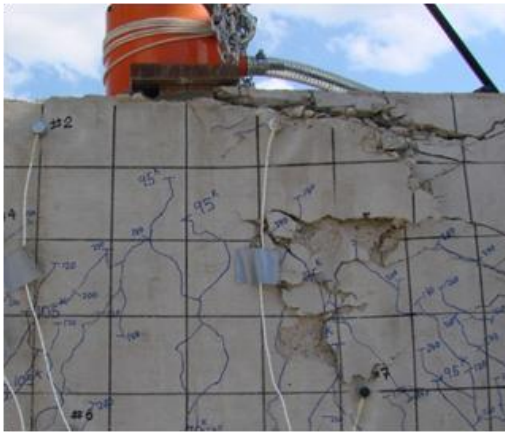
Figure 5.34 Typical Photos during Testing of SFRPC#2-1 Specimen: (a) Prior to Failure, (b) at Failure and (c) Crushing in Compression Zone
