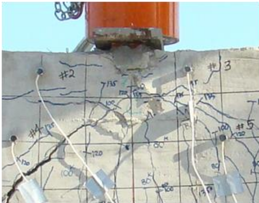
Figure 5.41 Typical Photos during Test of SFRPC#2-2 Specimen: (a) Prior to Failure, (b) at Failure, (c) Crushing in Compression Zone
