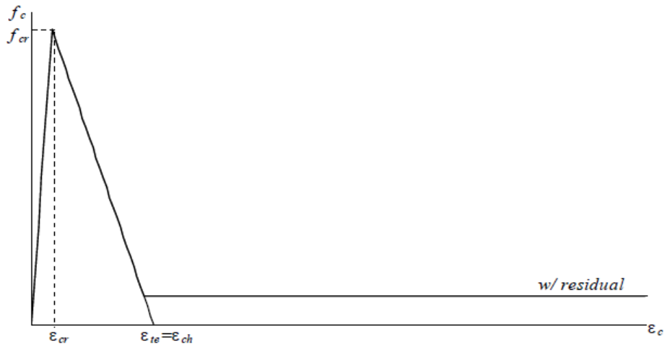
Figure 7.5 Linear Tension Softening Response with and without Residual [Wong and Vecchio, 2002]
