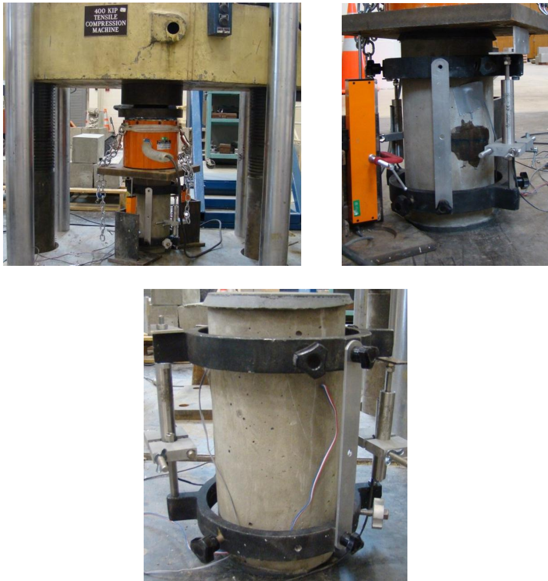
Figure 2.30 Test setup for obtaining Compressive Stress-strain relation
