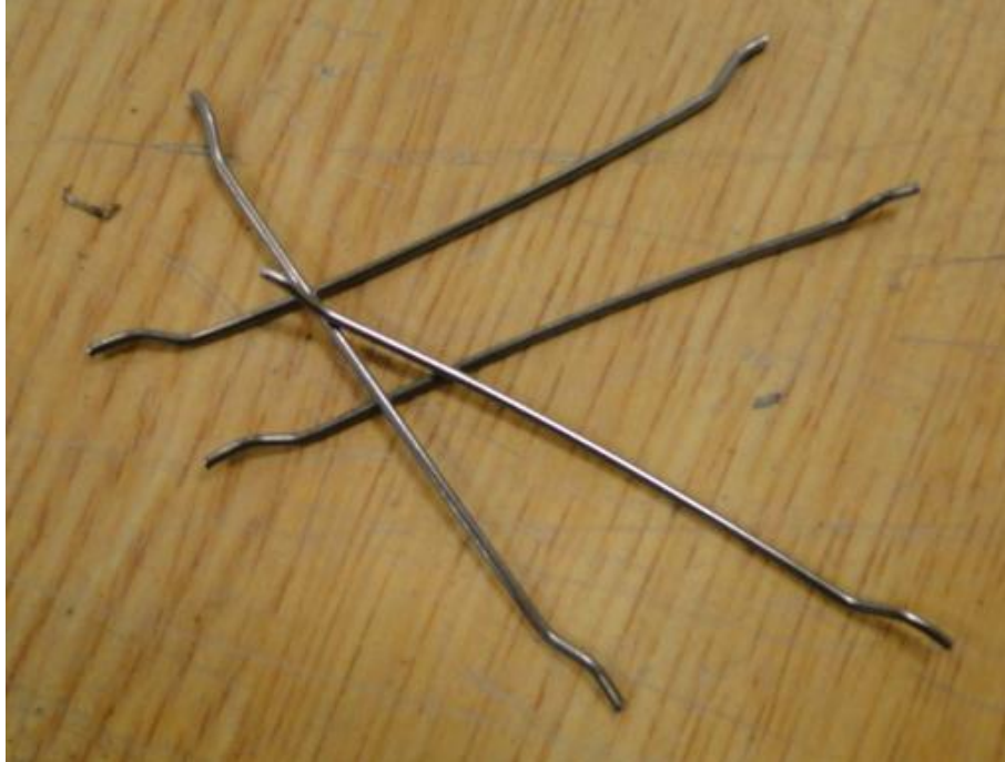
Figure 4.13 Steel Fiber Used in Further Study Type 5: Maccaferri Long Steel Fiber (Double Bend Hook at End, FF 3)
