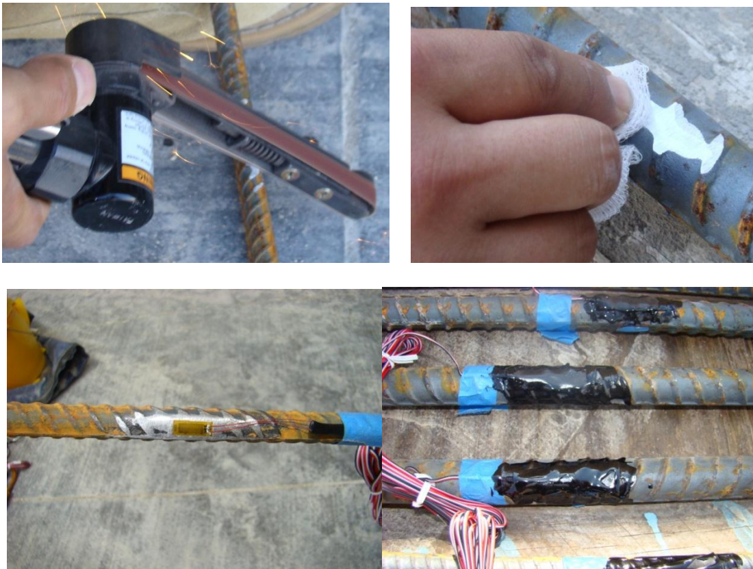
Figure 3.6 Example of Steel Strain Gauge Installment
