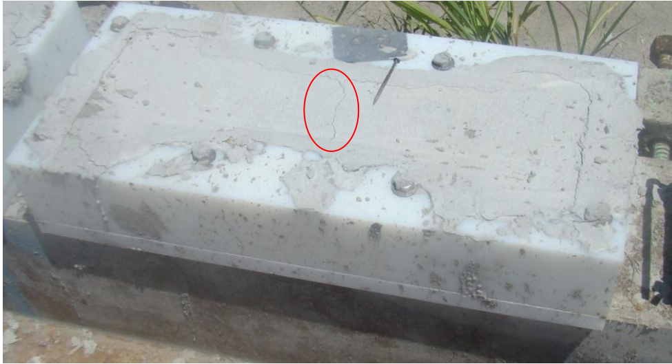
Figure 3.42 Typical Example of Problem with Preparation Dog Bone Specimens
