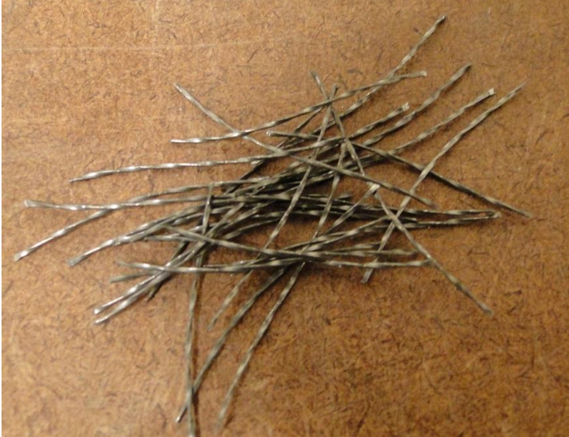
Figure 4.14 Steel Fiber Used in Fifth Phase of Study Type 6: Twisted Steel Fiber
