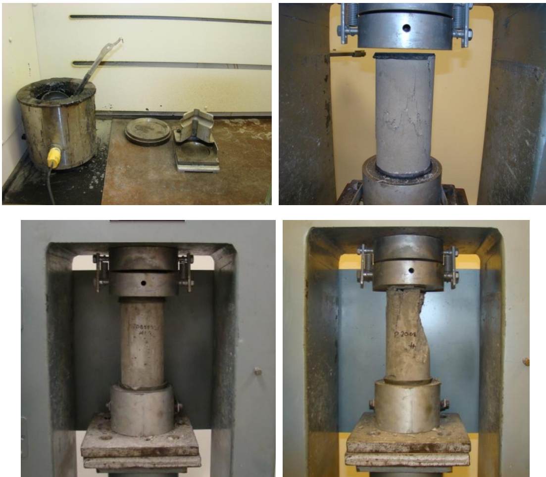
Figure 3.38 Typical Photos of Compressive Strength Test (Cylinder Test)
