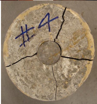
Figure 6.10 Typical Tested Photos Showing Radial Cracks
