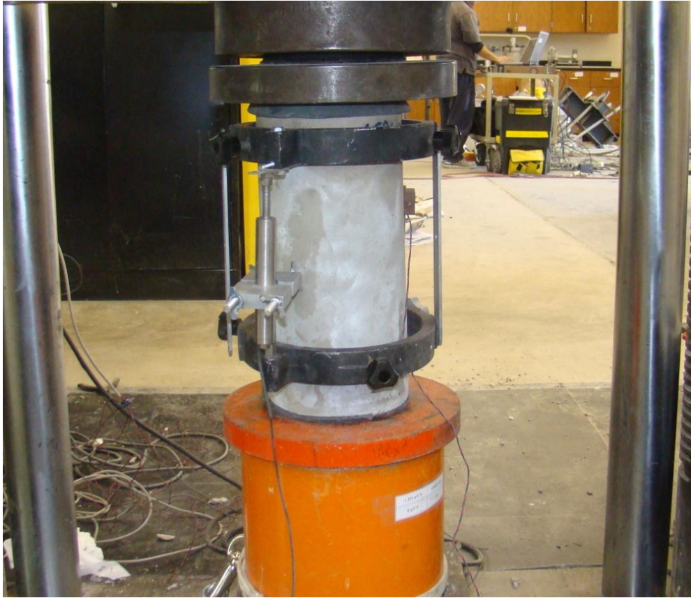
Figure 3.39 Testing Setup for Compressive Testing of Large Cylinders (6 × 12 inches)
