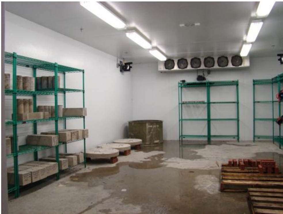
Figure 4.4 Preparation and Placing Specimens in Curing Room
