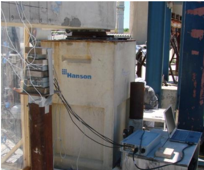
Figure 3.34 Acoustic Emission Sensors and Scanner Used in Second Phase Experiment
