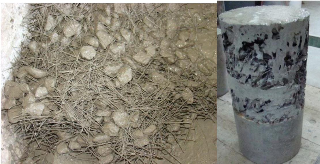
Figure 4.9 Example of SFRC Mix Problem (observed During First Phase) with Higher Volume Fraction of Steel Fiber
