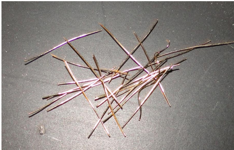
Figure 4.15 Steel Fiber Used in Fifth Phase of Study Type 7: Maccaferri Micro Steel Fiber
