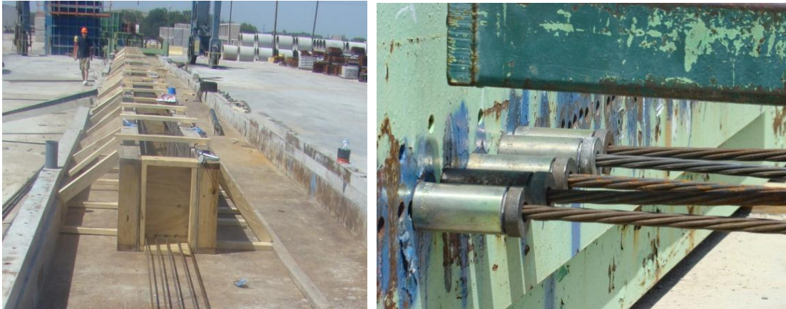
Figure 3.1 Pre-stressing Bed and Jacking in local precast plant (Hanson Pipe & Precast Plant, Grand Prairie, Texas)
