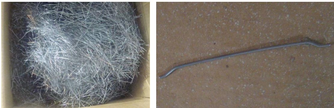
Figure 3.23 Type of Steel Fiber Used: Macceferri Long (FF3)
