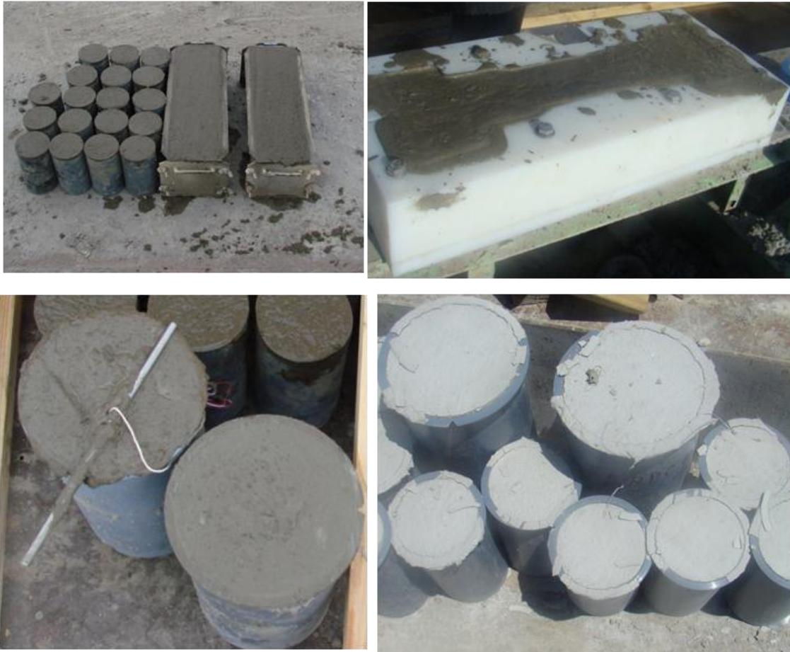
Figure 3.37 Typical Photos of Preparation of Specimens for Material Test
