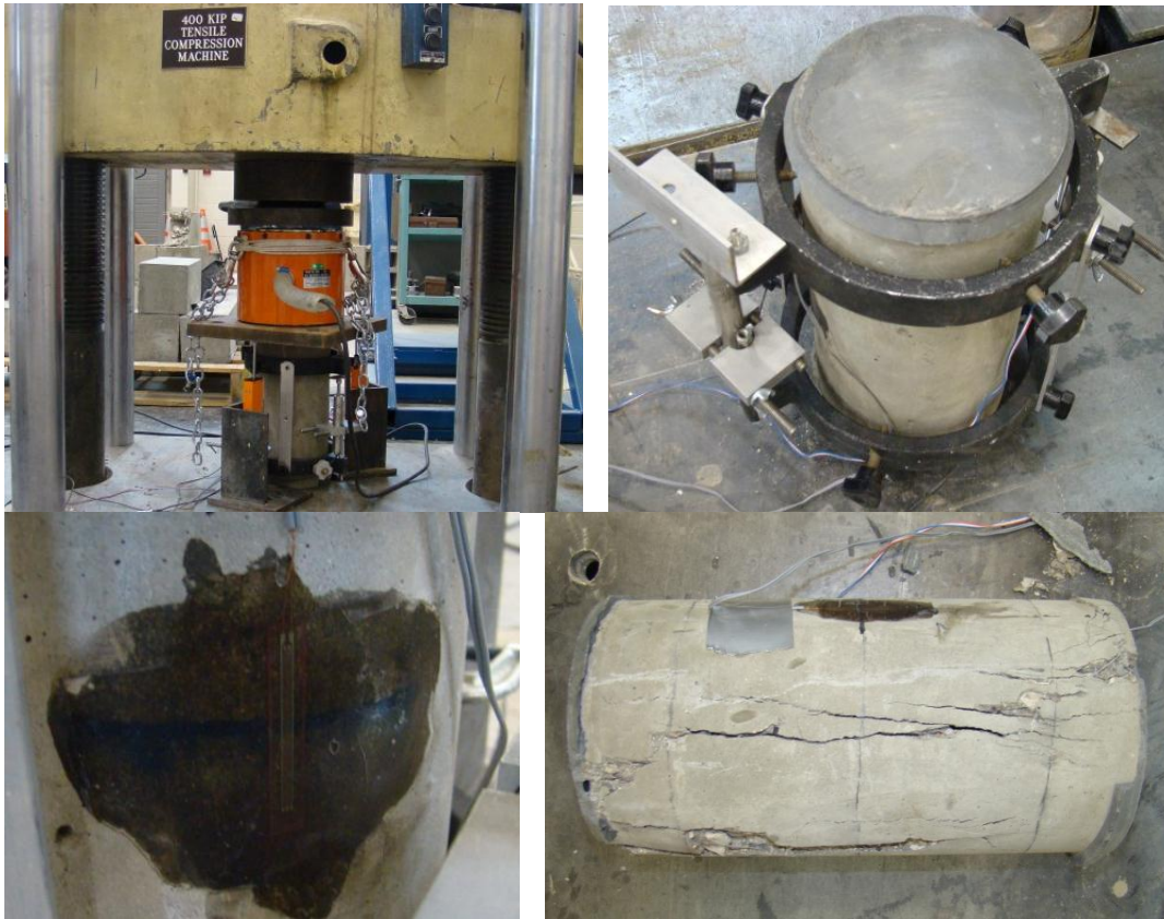
Figure 3.40 Typical Photos of Compressive Testing of Large Cylinders (6 × 12 inches)
