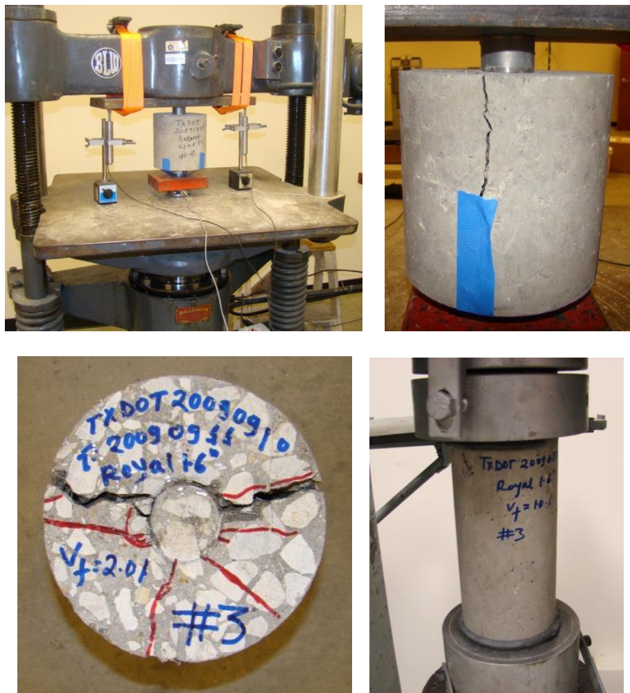
Figure 4.8 Typical Examples for Testing of Specimens (DPT and Compressive Strength)
