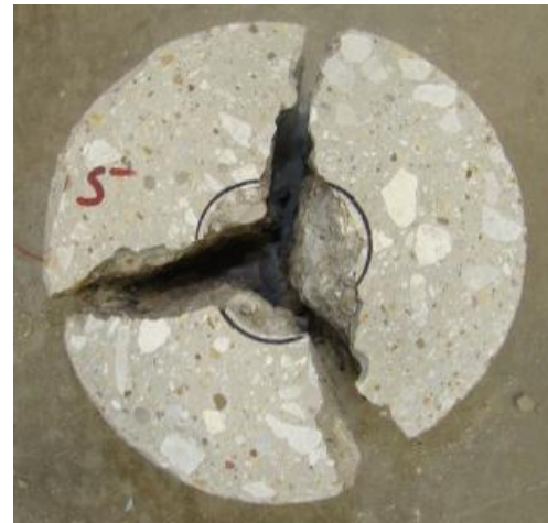
Figure 3.43 Typical Photos from Double Punch Test
