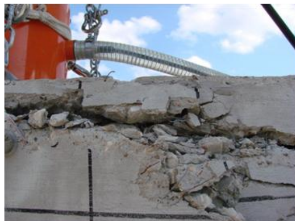
Figure 5.34 Typical Photos during Testing of SFRPC#2-1 Specimen: (a) Prior to Failure, (b) at Failure and (c) Crushing in Compression Zone
