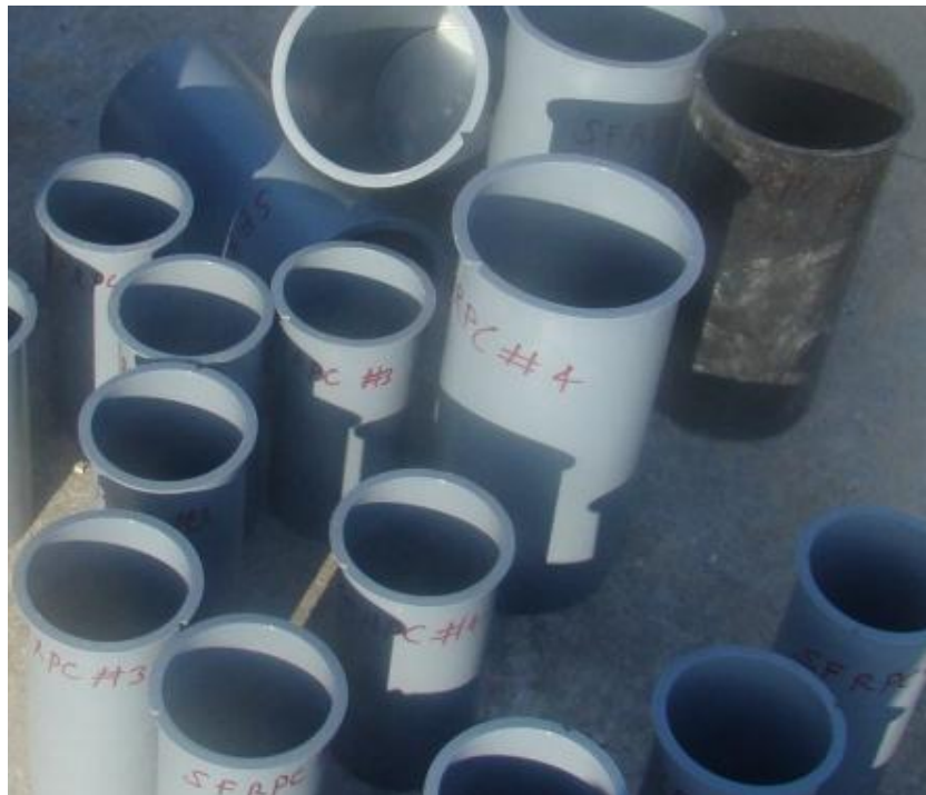
Figure 3.36 Preparations of Molds for Material Test Specimens
