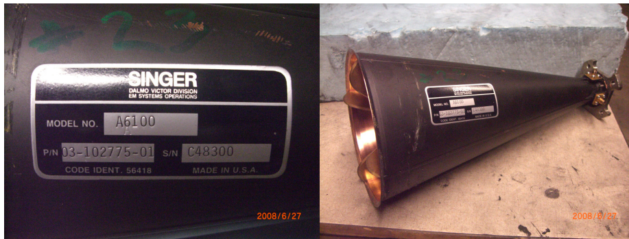
Figure 3.6: Probe antenna used in the measurement (Singer horn antenna model no. A6100).
