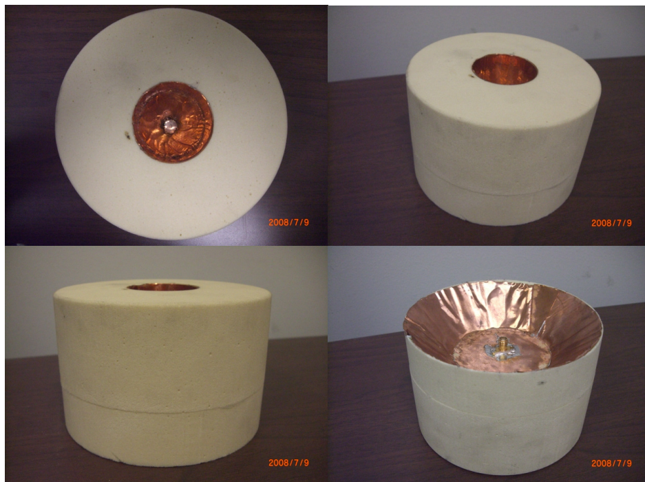
Figure 3.4: Cylinder-cone shape cavity quasi-planar conical antenna with bended ground plane.
