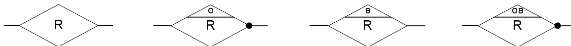
Figure 3.4. EER notation for unordered set, ordered set, unordered bag and ordered bag relationships (from left to right).
