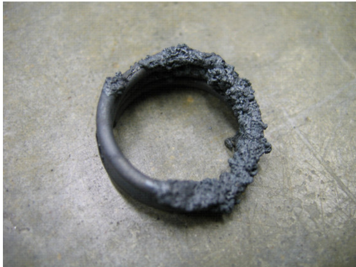
Figure 5.6 Fragment of a Shchelkin spiral after testing the PDE Mark 1.
