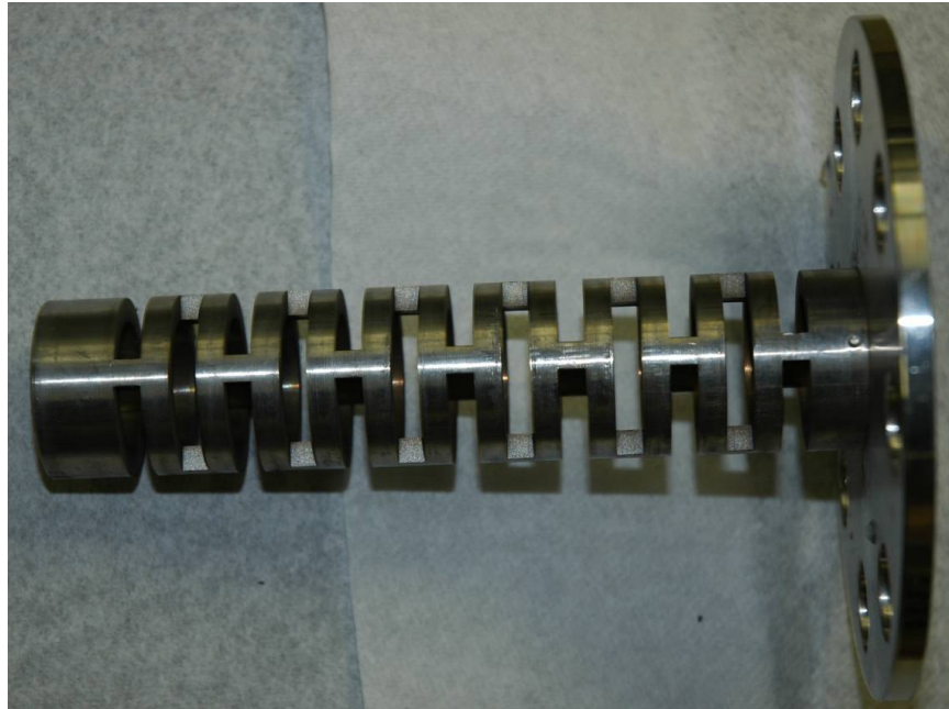
Figure D.7 Detail of the slotted-sleeve DDT device used in the PDE Mark 2.
