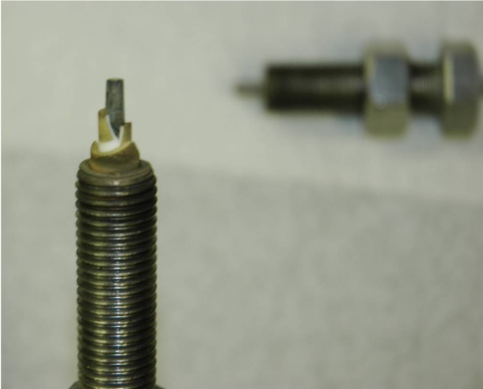
Figure D.6 Detail of the ignition plug used in the PDE Mark 2 shown after testing. Significant damage was sustained in a test lasting 15 to 20 s.
