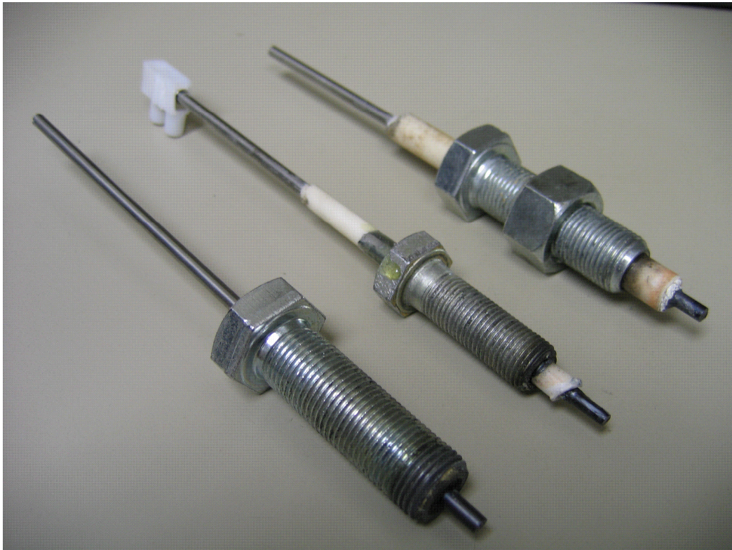
Figure 7.8 The electrodes used for HE and HVLE ignition on the PDE Mark 1 and the PDE Mark 2 suffered erosion as a result of the detonation. The electrode in the center is the HVLE electrode, while the electrode on the left hand side is the ground electrode. The erosion is obvious when one compares the shape of the two ends of the tungsten rods.
