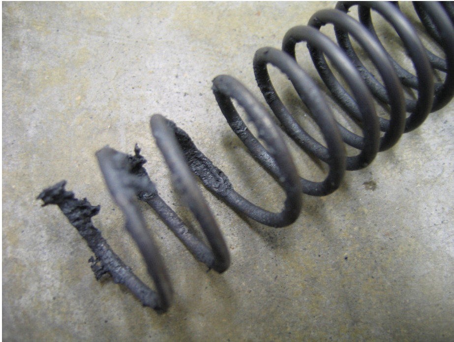
Figure 5.5 A sample Shchelkin spiral after testing in the PDE Mark 1 showing evidence of massive wear and deformation.
