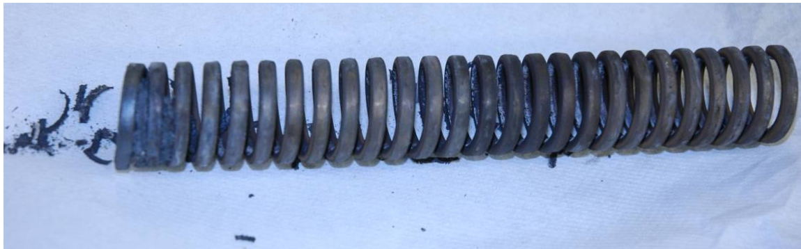
Figure D.4 Detail of a Shchelkin spiral that was tested in the PDE Mark 2 using stoichiometric propane-oxygen mixtures at 15 Hz for about 15 to 20 s. The spiral experienced significant damage.
