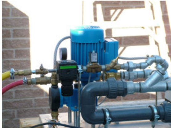
Figure 2.4 Equipment used to Control Foam Mix
