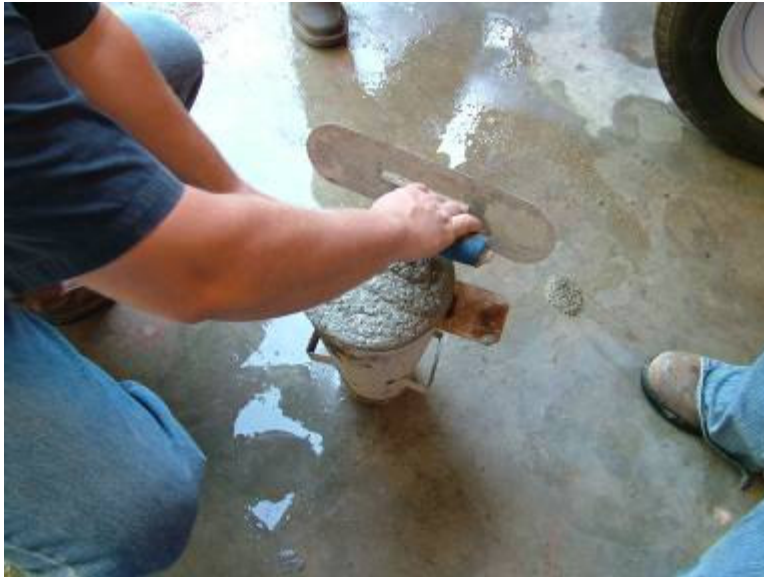
Figure A.1 Slump Test
