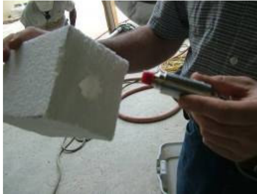
Figure 3.2 Foam Cover for Pressure Transducer
