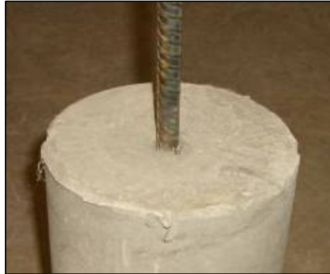
Figure 2.15 Specimen used for Pull-Out Strength Test
