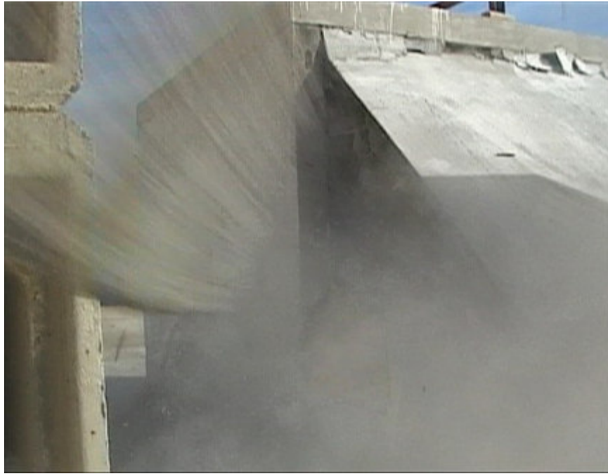
Figure 4.16 Failure of Wall Sequence 4
