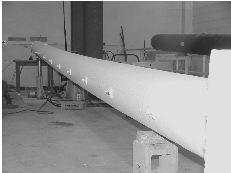
Figure 2.11 FRP pole deformed at 1 kips (4450 N)
