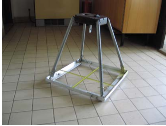
Figure 5. Photograph of the “tetrapod” fitted with a centimeter scale that was used in this study. Camera was attached close to the top of the tetrapod, at a fixed focal distance. The camera display was visible through a square hole in the top part of the tetrapod.
