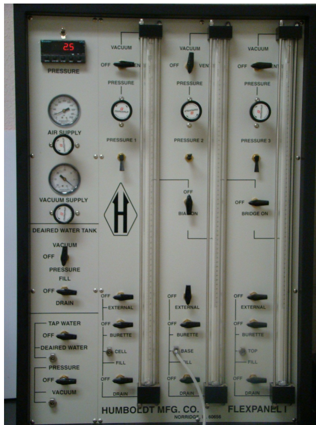
Figure 3.28 HM - 4150 – Model Pressure Control Panel
